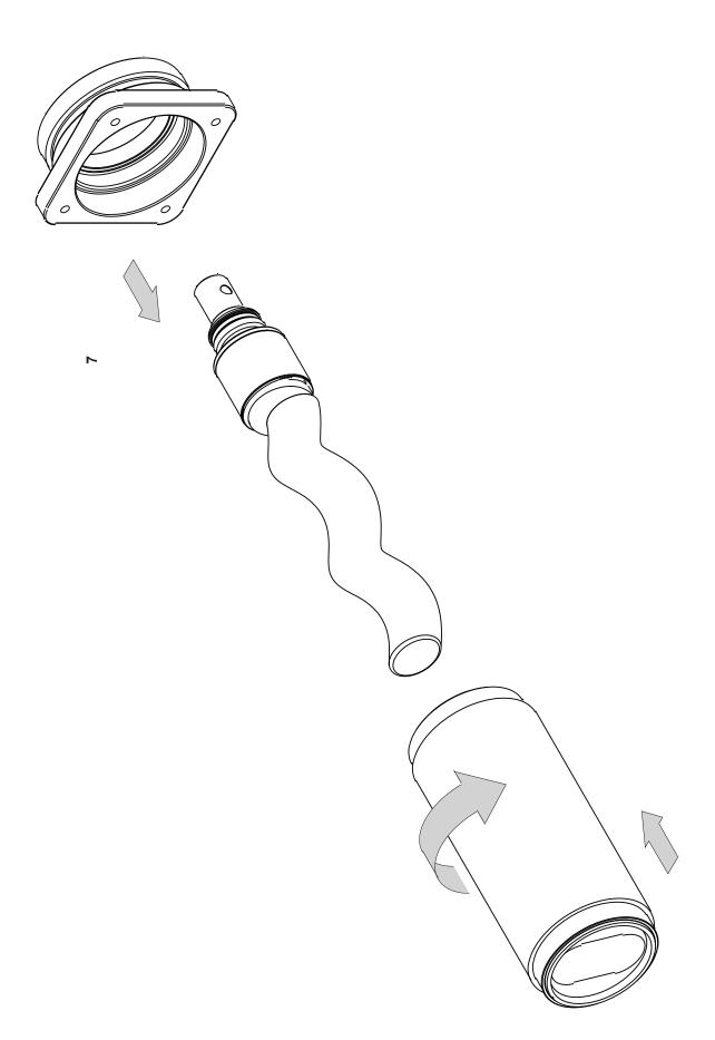
ROTOR & STATOR CHANGE ASSEMBLY
