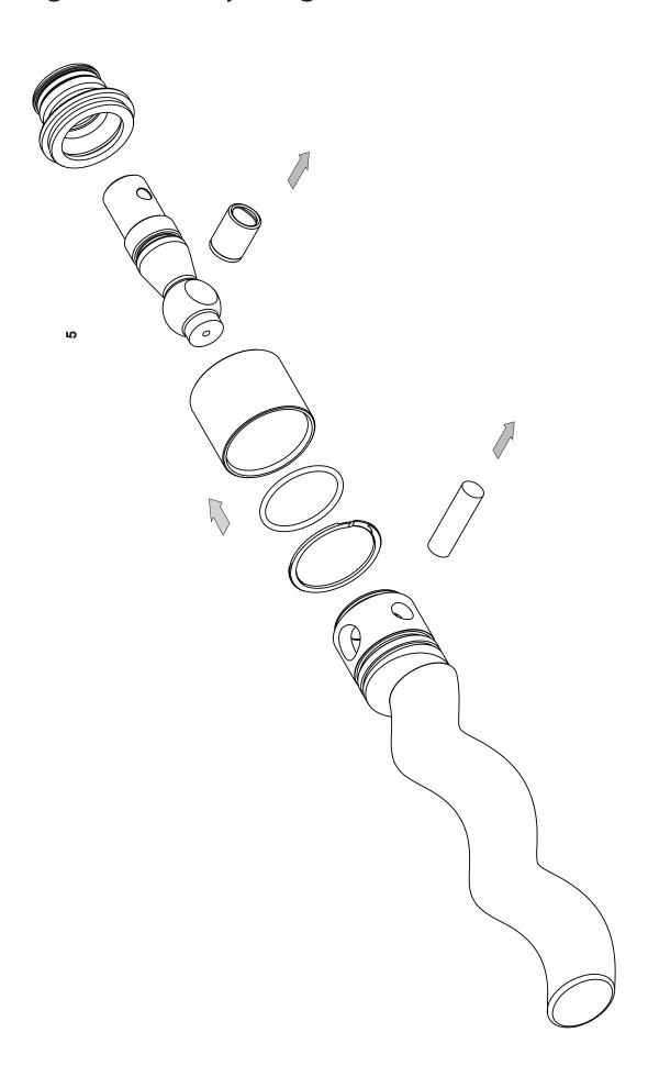
ROTOR & STATOR CHANGE DISMANTLING
