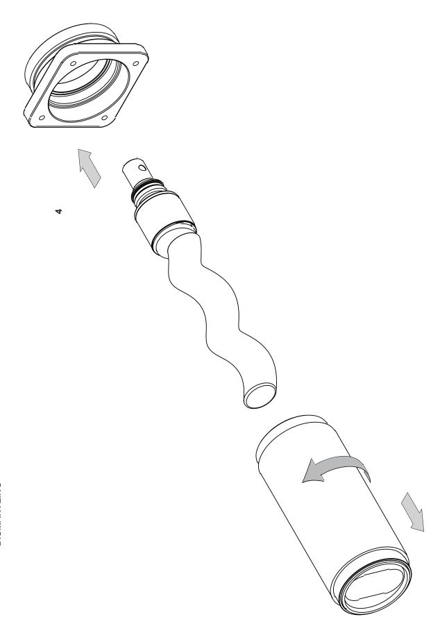
ROTOR & STATOR CHANGE DISMANTLING
