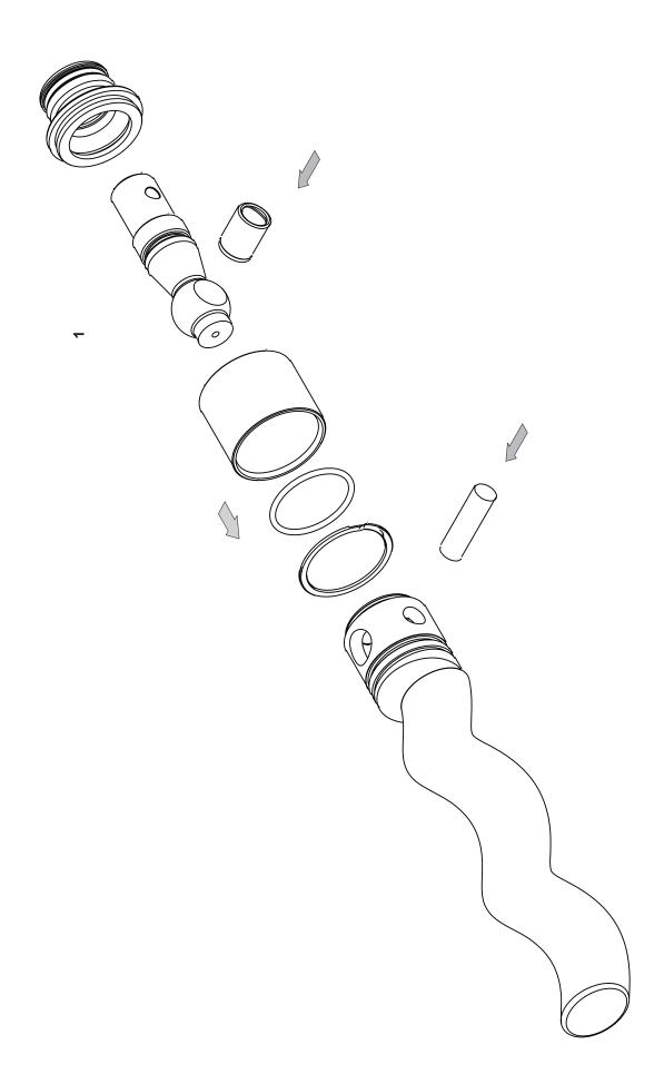
ROTOR & STATOR CHANGE ASSEMBLY
