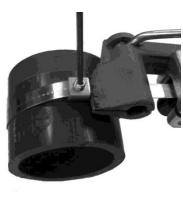
2. After tension is applied, insert set screw in Scru-Lokt buckle and tighten. To permit taking up Scru-Lokt clamp, or to re-use, a 3 inch (7.5 cm) stub should be left so that tool will be able to re-grip band later.
