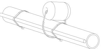
The power cable should be attached to the discharge pipe work with cable ties, and then fixed to the floats supplied with cable ties, as shown below.
