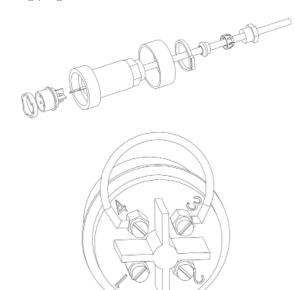
The SMC will only operate when pins 3 and 4 of the float switch are connected. The blanking plug contains a link wire
