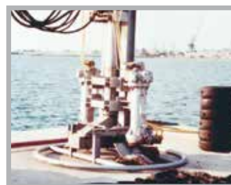
Barge emptying pump for oil based drilling mud and cuttings containing 'tramp' solids
