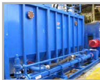
High Pressure hydro-cyclone feed for mud cleansing
