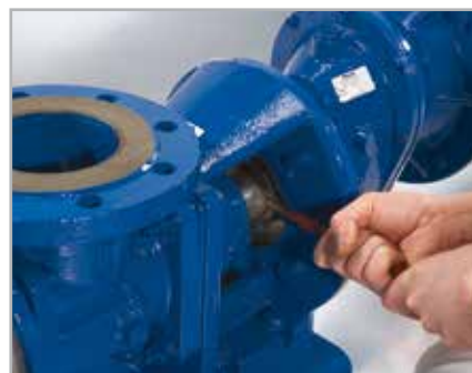
5. Pull back thrower guard and push pin out from the stub shaft
