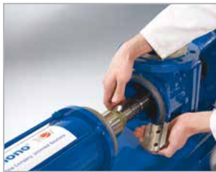
5. Pull back thrower guard and push pin out from the stub shaft
