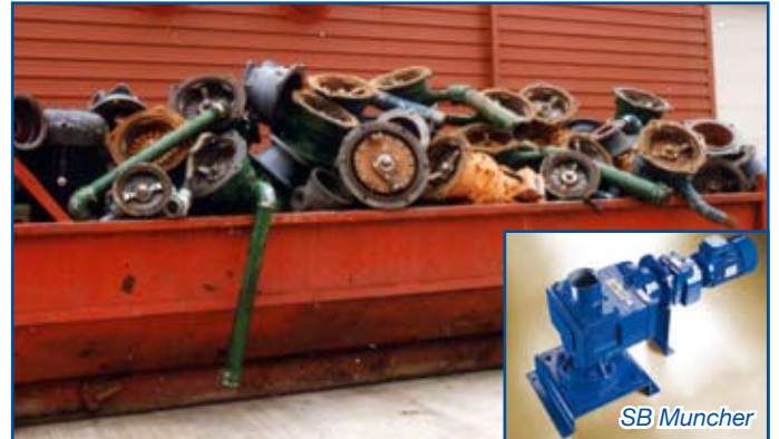
Some of the high speed macerators replaced with SB Munchers and Tri-Hammer macerators
